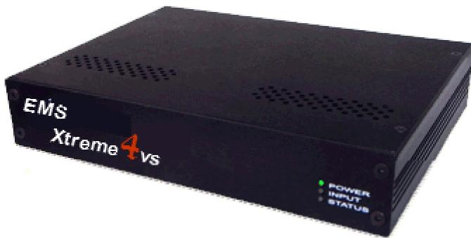
The EMS Xtreme4vs is a stand alone display wall controller that accepts a single or dual-link DVI input and can flexibly display this across four output monitors.
