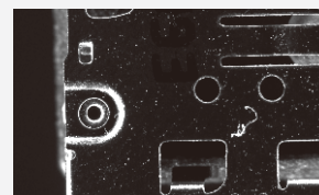
Shielding cover hole positioning detection
