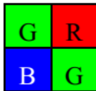
Figure 3-3 Bayer GR Pixel Pattern
